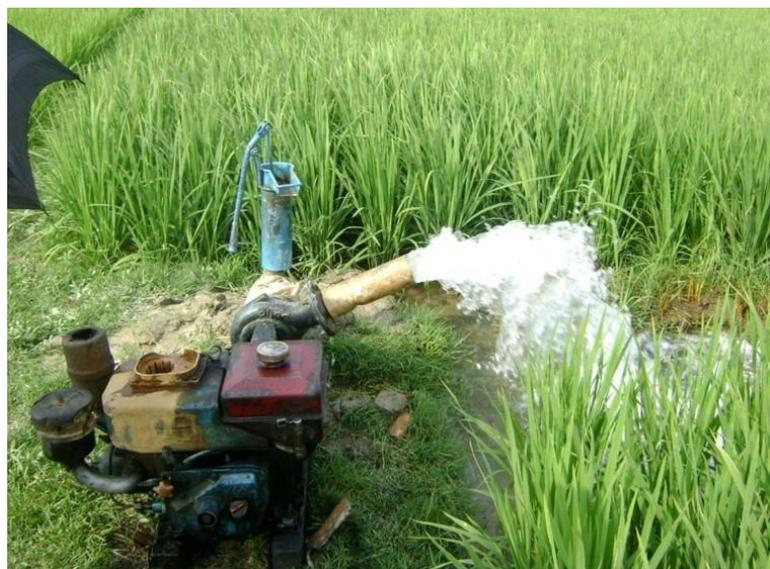
Figure 2 A STW pumping groundwater to irrigate rice field
